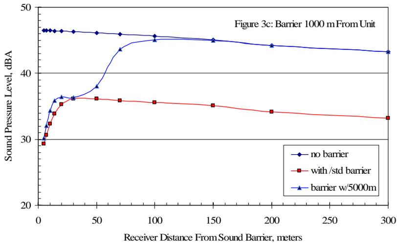
Figure 3: Sound pressure level as a function of distance from a residential barrier with a barrier height of 6 m for three different distances between the Unit and the barrier.
