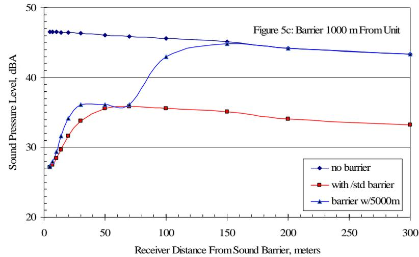
Figure 5: Sound pressure level as a function of distance from a residential barrier with a barrier height of 9 m for three different distances between the Unit and the barrier.
