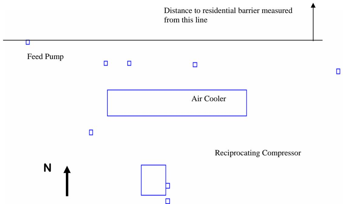
Figure 2: Sketch showing the location of noise sources modeled, and how the distance between the Unit and the residential barrier was measured.
