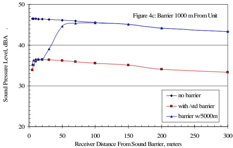
Figure 4: Sound pressure level as a function of distance from a residential barrier with a barrier height of 4 m for three different distances between the Unit and the barrier.
