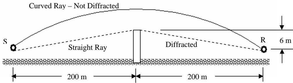
Figure 1: A barrier showing both straight and curved rays. The straight ray (when shown in a plan view) is diffracted, and has a computed IL of 8.5 dB, while the curved ray arcs over the top of the barrier with no IL.
